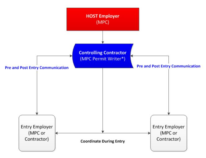
The above diagram shows the information and the coordination between the Host, Controlling and Entry Employers \* Controlling Contractor may be assigned to a third party per site approval for Green Field/New Construction
