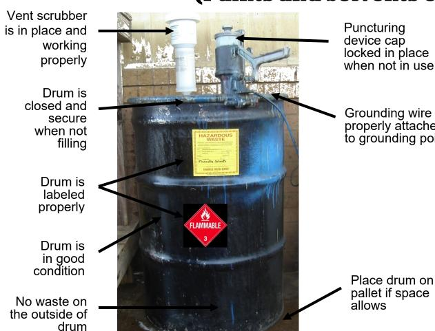
Grounding wire is properly attached to grounding point
