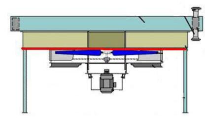
The Red Line indicates the confined space plane. All work above the red line (fan hub) will require confined space entry. All work on or below the Fan hub (Fan blades, motor, pulleys, gearbox) will **NOT** require confined space entry.
