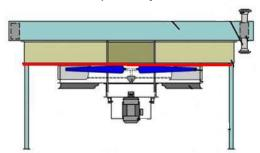
**IMPORTANT**: The Red Line indicates the confined space plane. All work above the red line (fan hub) will require confined space entry. All work on or below the Fan hub (Fan blades, motor, pulleys, gearbox) will NOT require confined space entry.
