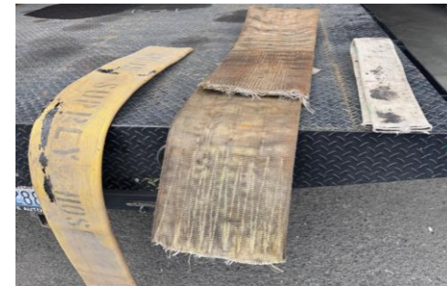
Sharp edge of motor that caused rigging damage
