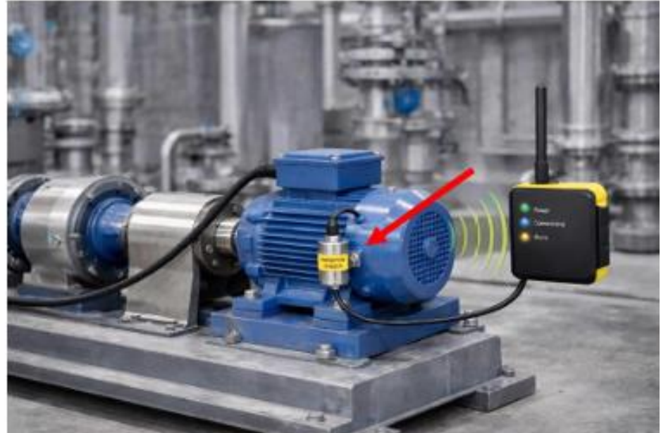
Figure 1. Motor with vibration sensor installed. Image generated with the prompt 'Motor with vibration sensor installed' by OpenAI, ChatGPT, 2026.
