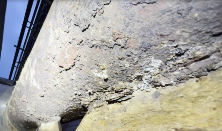
CUI scale can mask localized wall thinning
