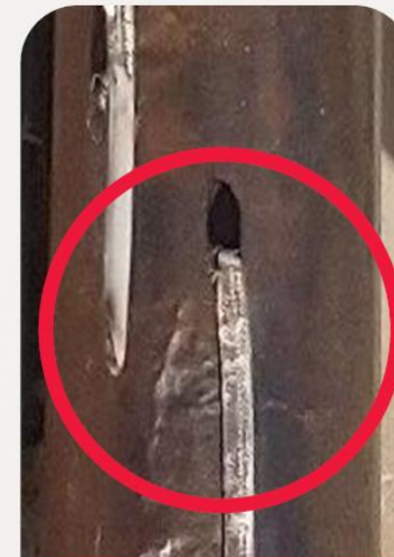
Damaged Electrical Heat Trace from an Angle Grinder
