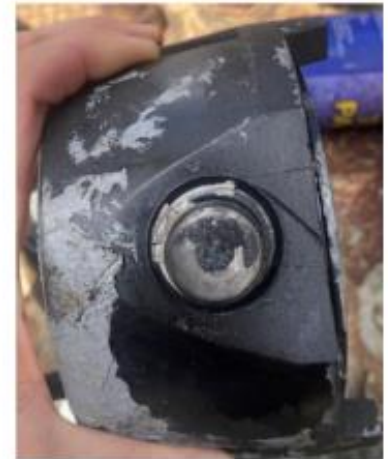
Figure 2. Plugged pressure gauge from the incident
